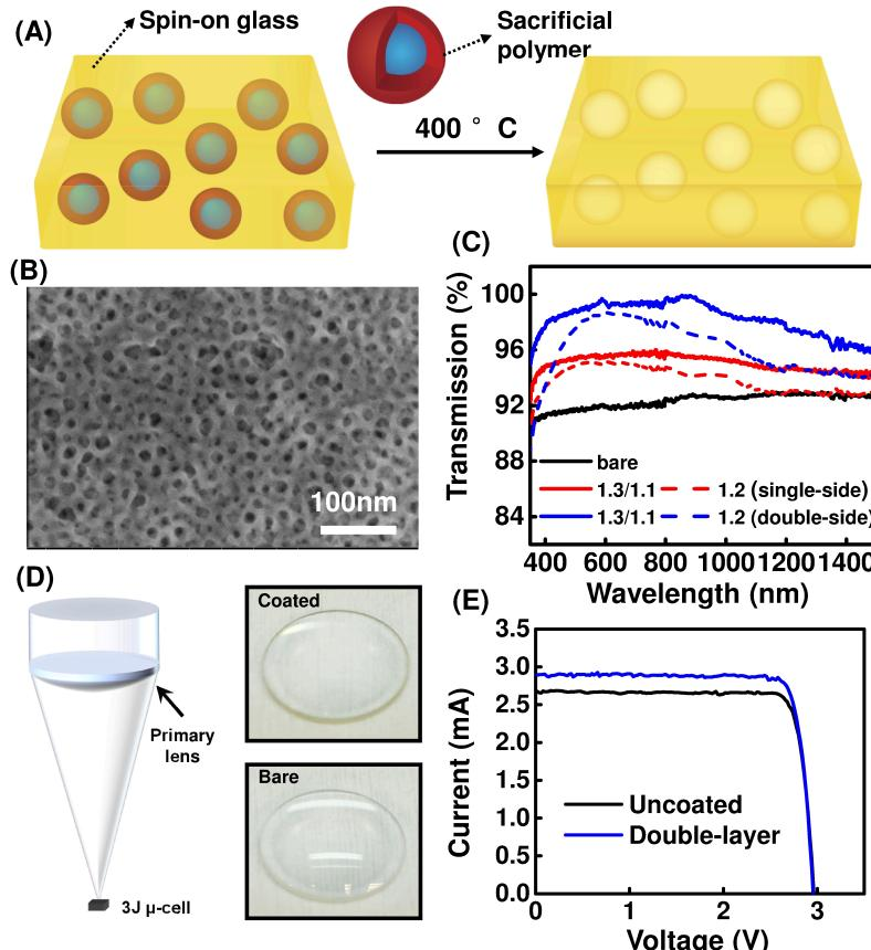
(A) Coating fabrication; (B) SEM image; (C) Transmission enhancements; (D) CPV setup and optical images of coated and bare lenses; (E) IV curves showing CPV performance enhancement.
